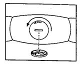
cover and turn the cover counterclockwise to the "open" position. Remove the cover.
